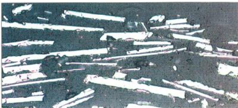
Fig. 7 - Cross section of test panel coated with naturally occurring MIO, MIO platelets exhibit a consistent tendency towards parallel to sub-parallel orientation with respect to the steel substrate.
