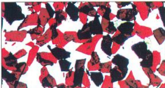
Fig. 5 - Naturally occurring MIO -53+38 micrometer fraction (oil immersion, transmitted light). Sample exhibits uniform content of thin lamellar micaceous iron oxide.
