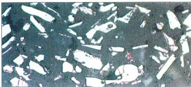
Fig. 8 - Cross section of test panel coated with synthetic MIO. Fine MIO platelets together with the more granular iron oxide components exhibit a more random orientation within the coating layer. Extended parallel or sub-parallel orientation of the MIO component was generally absent throughout all of the cross sections examined.
